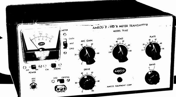
In response to the demand for an inexpensive VHF transmitter, Ameco has brought out its Model TX-62. It is a complete 6 and 2 meter, 75 watt phone and CW transmitter. The A-C power supply is built in. It is easy to tune. All circuits up to the final are broadbanded. Since the meter can read RF output, all one has to do to tune up the transmitter is to peak the final plate and loading capacitors for maximum reading.
